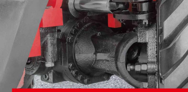
Oscillating steer axle allows either wheel to step over obstacles keeping the truck and load level.
