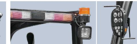
The new e<sub>c</sub>ciency ligh ting system employs LED illuminant and new type reflector to reduce energy consumption, improve significantly illumination performance and prolong work time.
