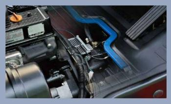
In addition to rubber damper between overhead and frames, compound engine damper and full floating power train achieve flexible connection between frames and driving system, as a result, traveling vibrations and vibrations from the driving system are significantly reduced.
