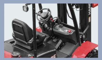
2. The extra foot space is provided to reduce operator fatigue significantly, non-slip step makes getting in and out easy and safe. The new designed steering wheel, new brake system and the easy-to-operate levers provide total handling operation.
