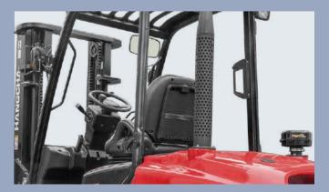
The new design mast provides broad forward visibility due to the longer distance between inside mast.
